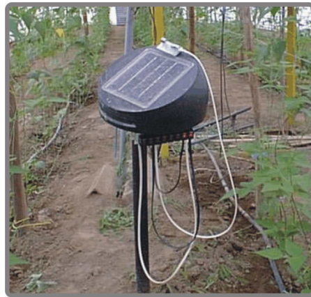
Fig.2 – Photograph of a SPWAS station inside a greenhouse.
